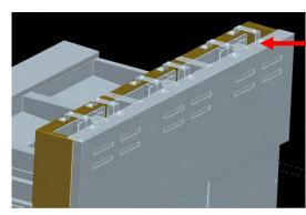
STEP 1: INSTALL RISERS (2601156) TO FLUE
