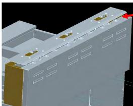
STEP 2: INSTALL COVER PLATE (2601155) TO RISERS USING CABINET SCREWS (8090434). ENSURE THE ANGLED SLOPE IS TOWARDS THE REAR OF THE FRYER. THE 90° BEND SHOULD BE FACING THE FRONT OF THE FRYER.
